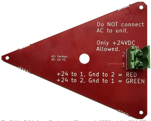
The AD-16 is a Bi-Color Lantern Direction Arrow. When you apply +24VDC to pin 1 it will light RED, and to pin 2 it lights GREEN. You can only used a regulated +24VDC power source. These are designed to fit into standard acrylic elevator hall lantern ADA lenses.
